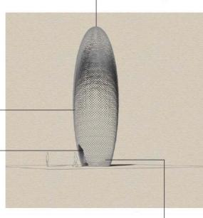
Polished aluminium "petals" attached to a steel framework.
