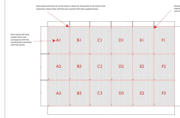
Example Installation Map – Please refer to project specific installation map which will be supplied in both a physical and digital copies. NB. We recommend making allowances for up to 0.5% difference of the dimension given due to material expansions. A level of flexibility on site may be required
